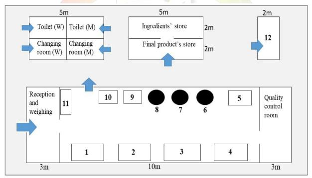
1: Selection/grading, 2: Washing/disinfection, 3: Peeling/slicing, 4: Juice extraction/filtration, 5: Juice clarification, 6: Refrigerator, 7: Electrical drier, 8: Autoclave/pasteurizer, 9: Sealer/capper, 10: Packaging and labelling, 11: Double dishwasher, 12: Boiler room/solar driers.
